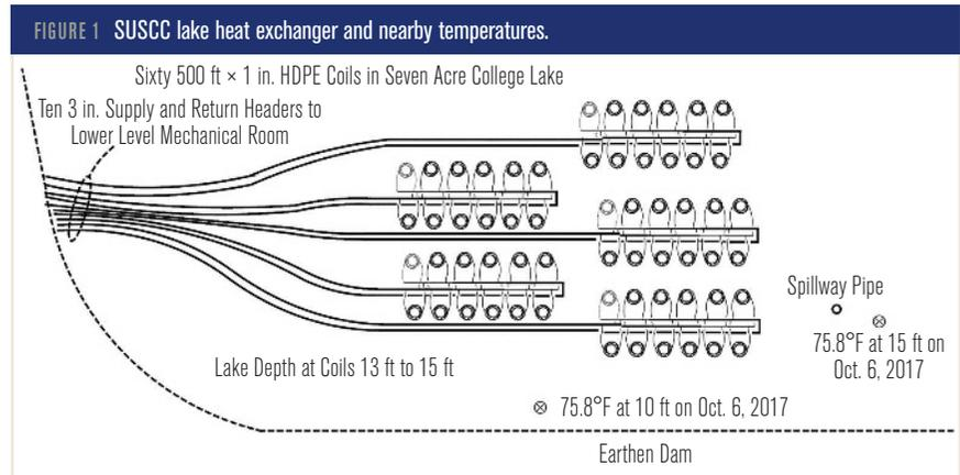
into place with a boat. The coils are located where the lake depth is 13 to 15 ft (4 to 4.5 m). The client reported that the lake level has remained relatively constant even during drought periods.
